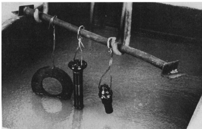
Figure 16. Molten salt is commonly used to heat and to quench high speed steel tools
