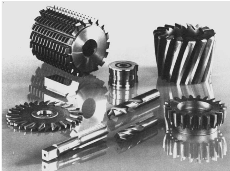
Figure 7. Drills, hobs, end mills, taps, formtools and milling cutters are typical cutting tools made from high speed steels
